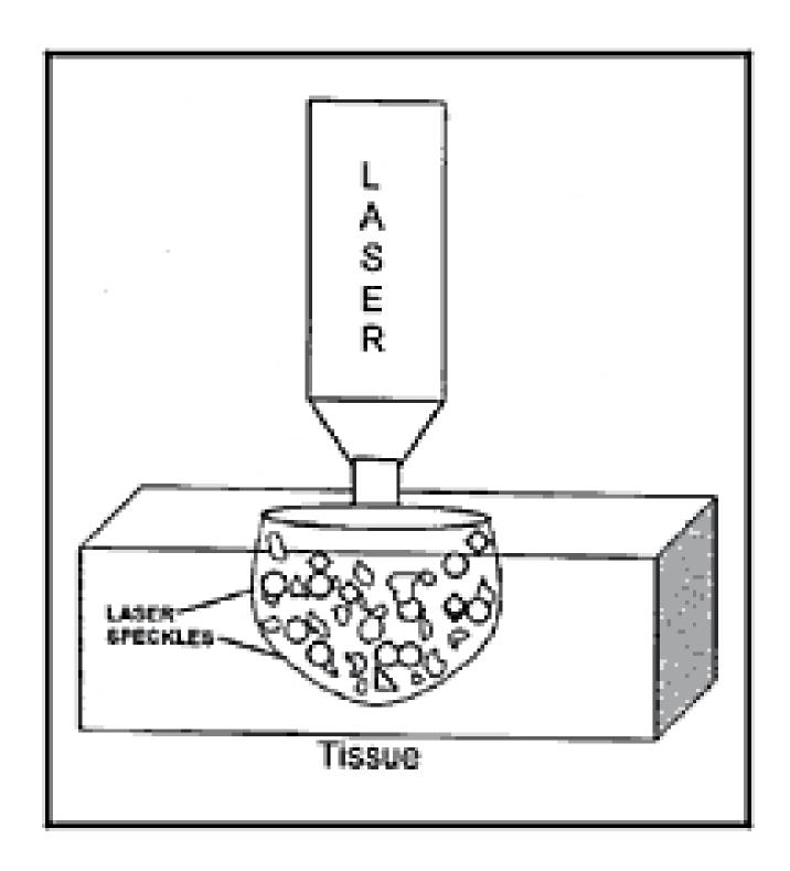
As a laser beam penetrates tissue, variations in optical density will bend portions of the beam. Speckles are regions where laser light is reinforced or weakened. *This uneven distribution of energy, unique to laser light, is dynamic and vibrant*. It is almost as if coherent light were alive. In contrast, if you shine a flashlight or LED against a wall or on a piece of paper, you will note that the energy distribution is flat and motionless.
